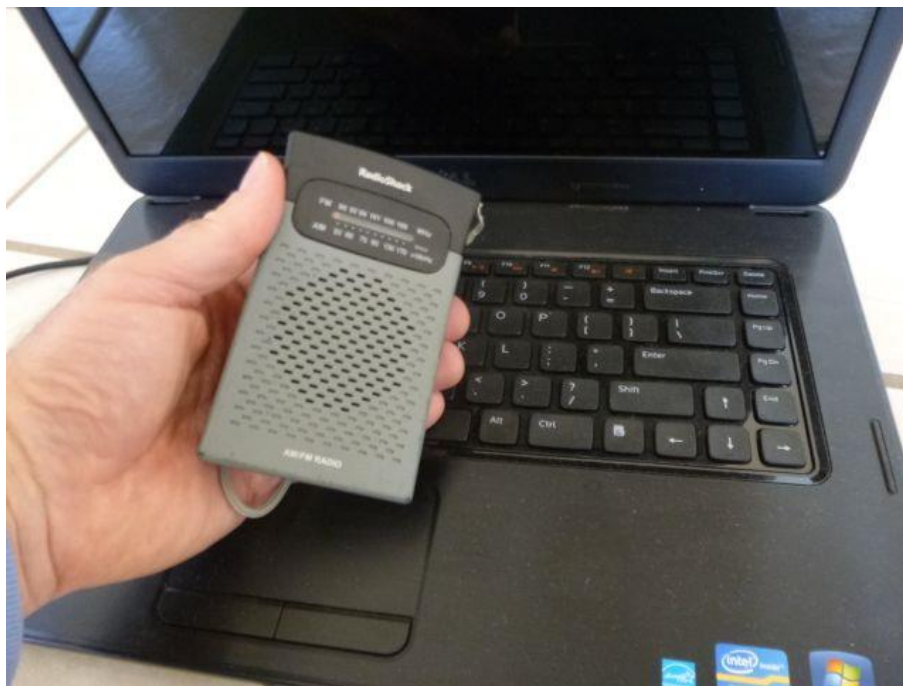
Any computer will generate a lot of static in an AM radio.
