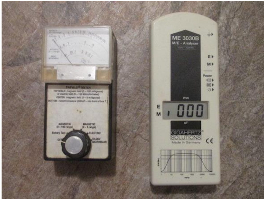
Two moderately priced gauss meters that are sufficient for most people's needs: Alpha Labs TriField (left) and Gigahertz Solutions ME 3039B (right).
