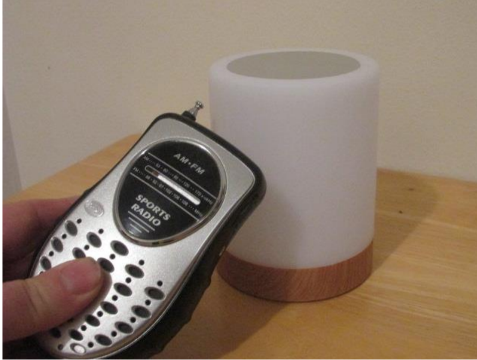
Checking a rechargeable night light that is controlled by touch. It radiates even when “off.”
