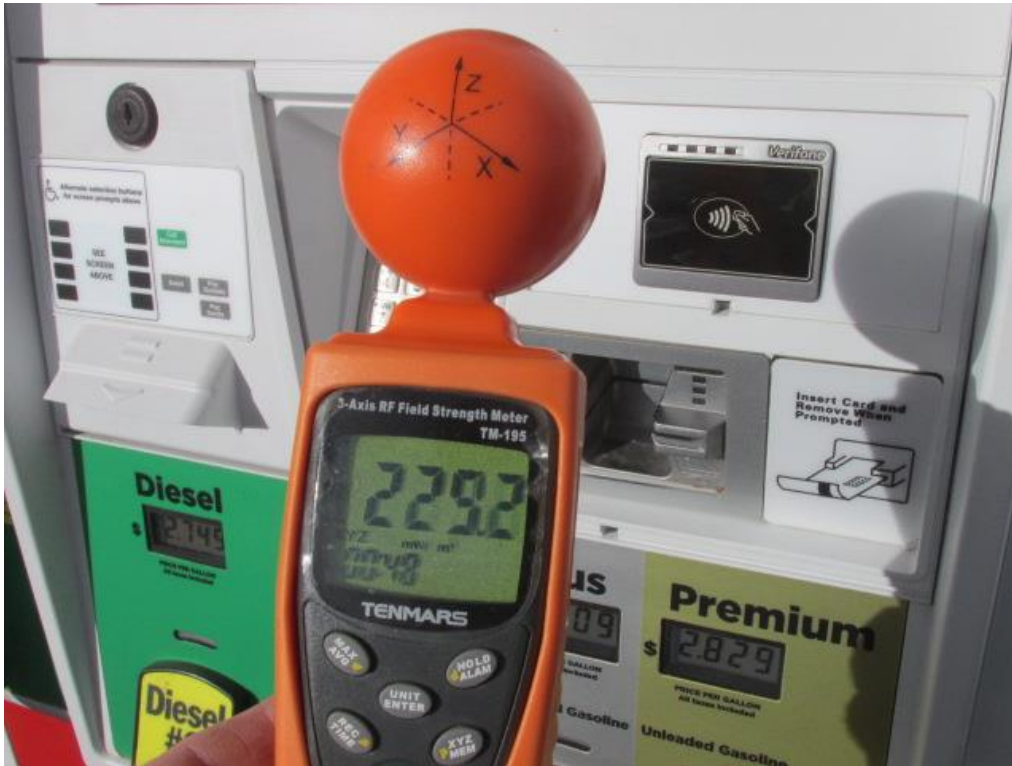
RF meter showing the radiation from a pump at a gas station. The pump has a wireless pay feature that radiates whether used or not.
