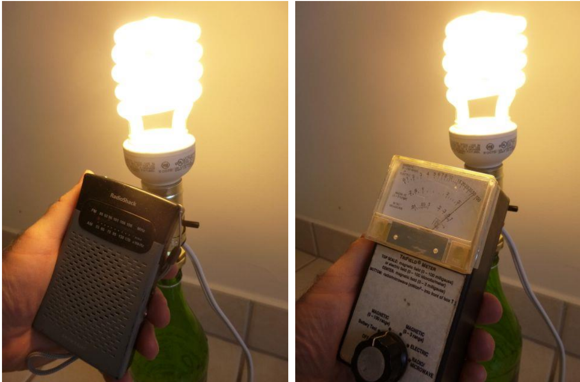
Measuring a compact-fluorescent light bulb with both an AM radio and a gaussmeter. The bulb emits a wide range of frequencies picked up by both instruments.
