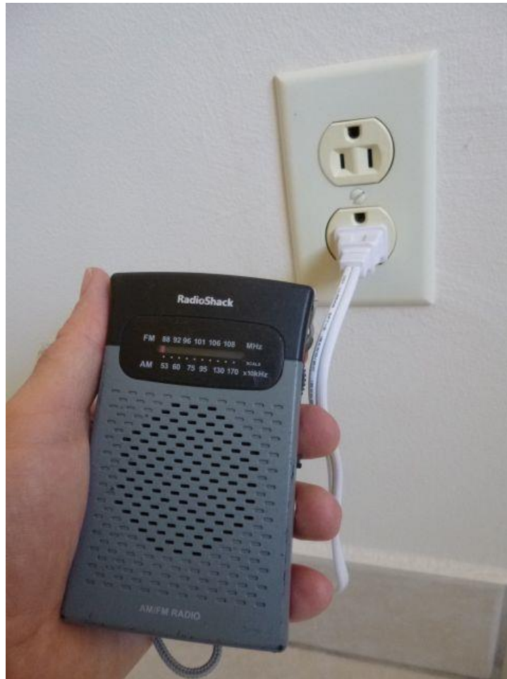
Measuring dirty electricity with an AM radio.
