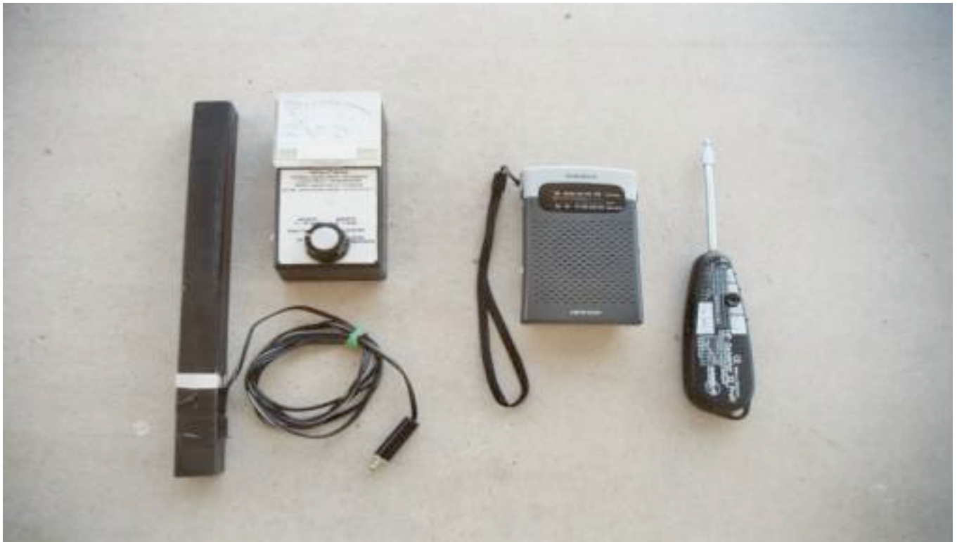
Instruments for measuring electromagnetic fields (EMFs) Left to Right: upgraded Trifield gaussmeter, AM radio, HF Detektor
