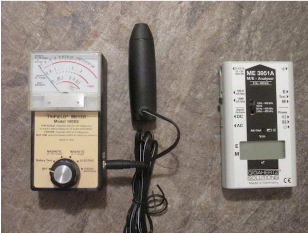
Two very sensitive gauss meters that can detect EMF down to 0.001 milligauss (0.1 nanotesla): Alpha Labs TriField 100XE with external probe (left) and Gigahertz Solutions ME 3951A
