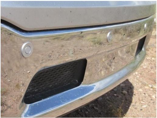
Circular radar transmitters embedded in a steel bumper. They can be hidden inside plastic bumpers.
