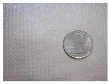
Perforated laminated aluminum foil. The tiny holes prevent mold by allowing the walls and ceiling to breathe.
