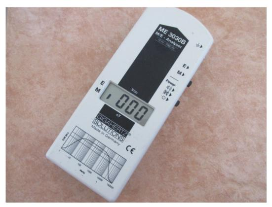
Instrument that can measure both the electric and the magnetic fields from household wiring. This instrument is sensitive down to 0.01 milligauss (1 nanotesla). It is pictured inside an ultra-low EMF house where the magnetic field is about 0.001 milligauss, so the instrument is unable to detect anything.
