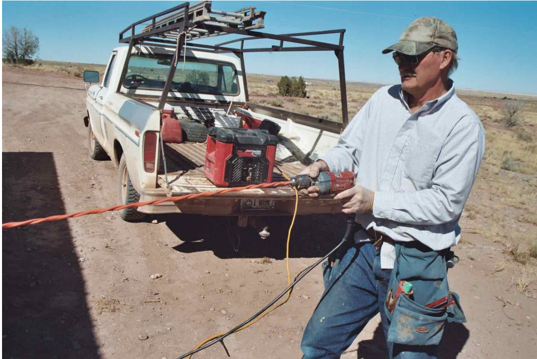
Twisting an electrical cable using a slow-moving variable-speed power drill.
