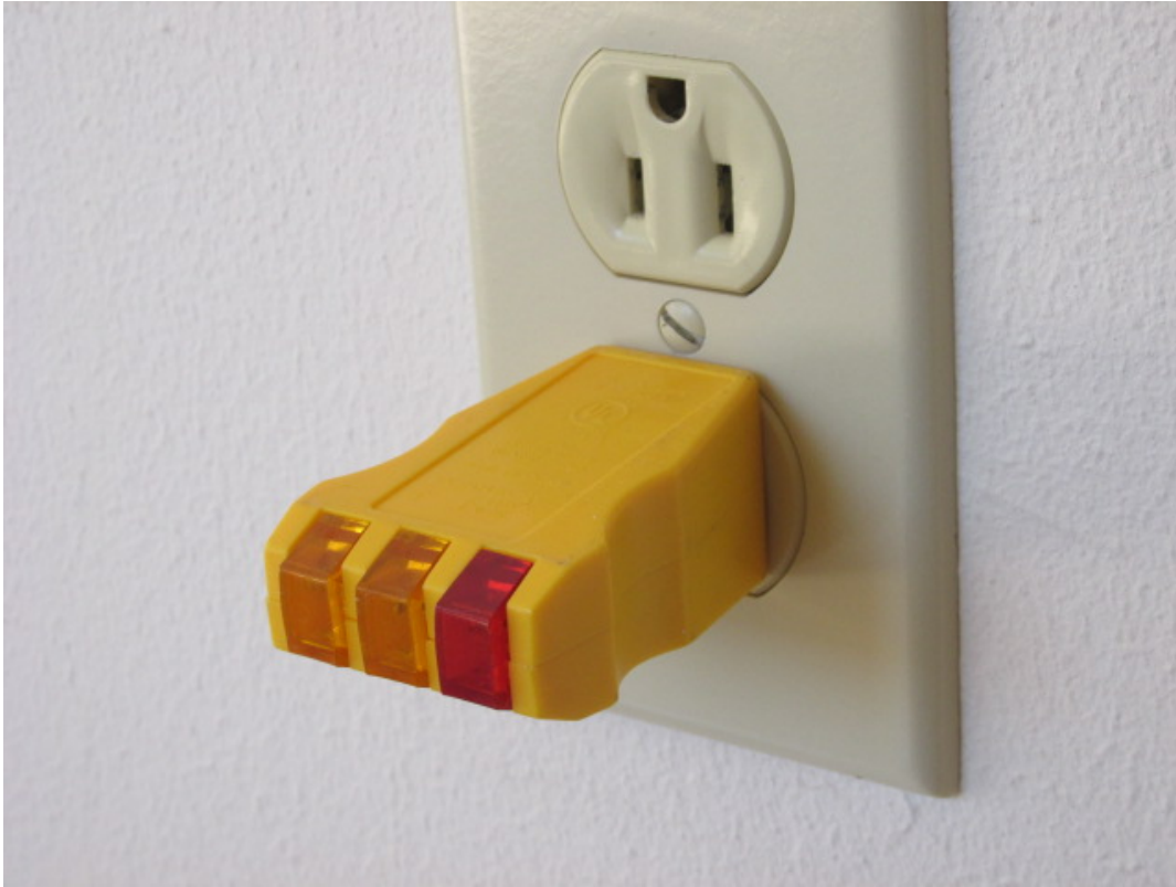
A simple low-cost outlet tester.
