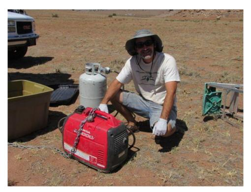
An off-gridder with a portable 2000 watt Honda EU2000i generator with optional propane kit.
