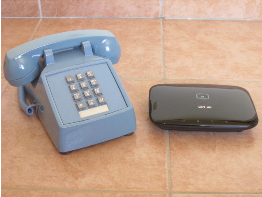
A fixed wireless device creates a “landline” where there otherwise isn’t one. The box on the right is the Verizon Home Phone Connect, which has no Wi-Fi or local network.
