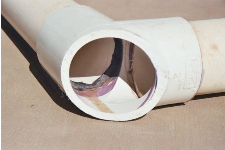
Cut-out PVC water pipe, showing excess glue exposed to the water stream. Note how the glue has leached along the bottom of the pipe.
