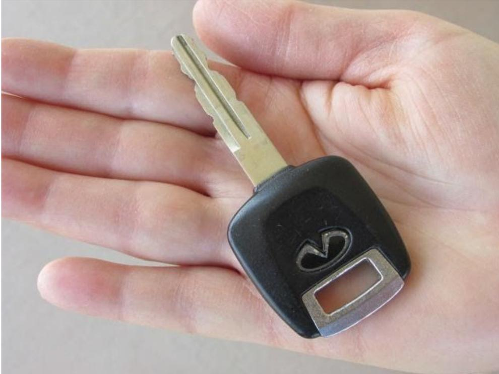
*An RFID key from a 2003 Infiniti G35.*
