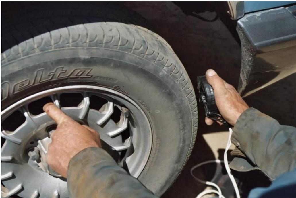
*Degaussing tire mounted on the car. One hand spins the tire while the other hand operates the degausser. It can be done by a single person, but it is harder to do the movements smoothly and with no stops.*
