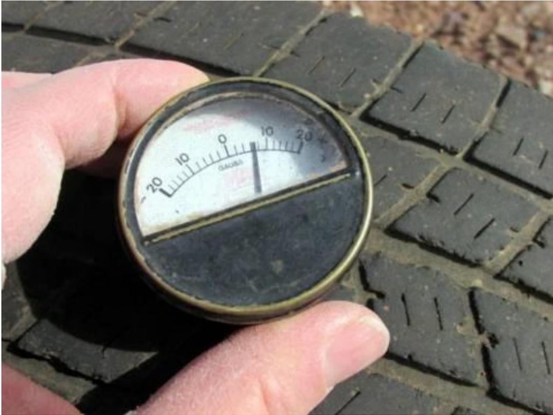
*Using a mechanical magnetometer on a car tire.*
