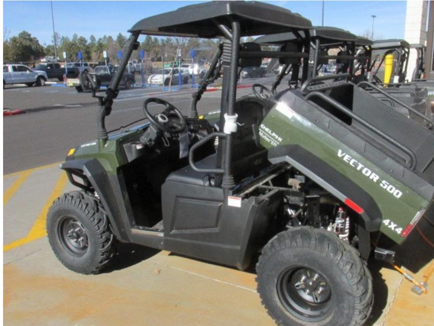
*A roundabout vehicle with the engine located inside the driver' seat.*
