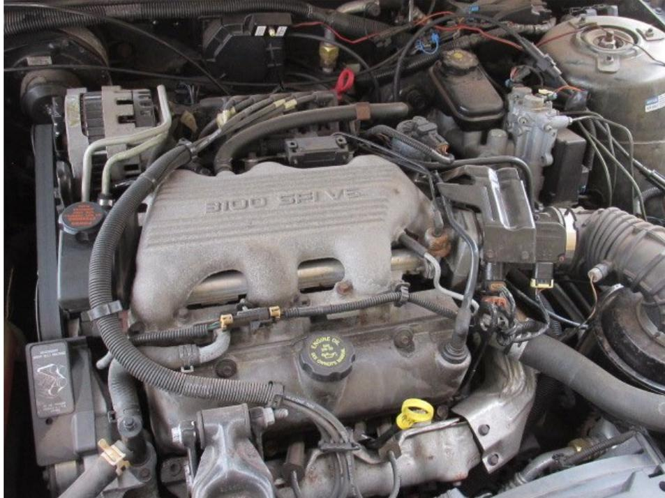
*Transverse mounted engine in a 1996 Buick, as seen from the front. The belt is on the side instead of in front. Note the alternator placed up against the firewall. The radiator fan is electric.*
