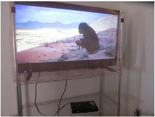
Television shielded with copper mesh in front of the screen. It can be seen as a reddish tint. It is less visible in a darkened room and on a larger screen.
