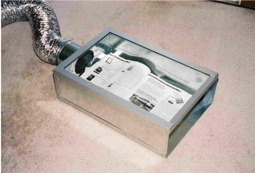
Vented reading box with one open side.
