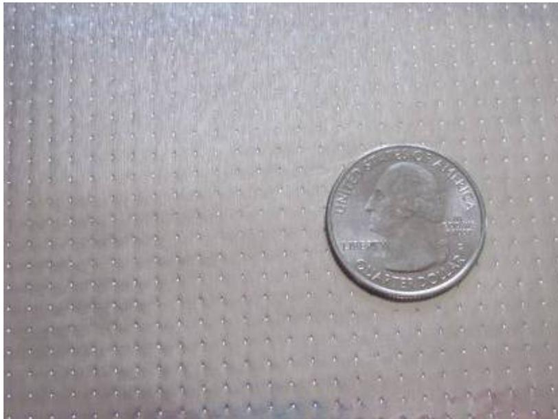
*Perforated laminated aluminum foil. The tiny holes prevent mold by allowing the walls and ceiling to breathe.*
