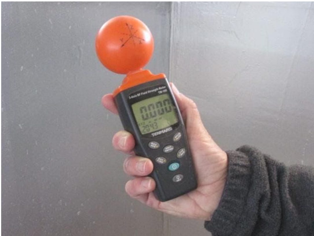
Measuring the microwave radiation inside a shielded room. Here the level is so low the RF meter can't detect it.
