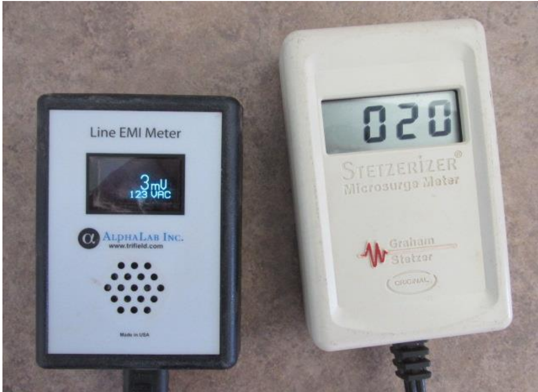
The same instruments showing clean power in a grid-connected home with no solar system.
