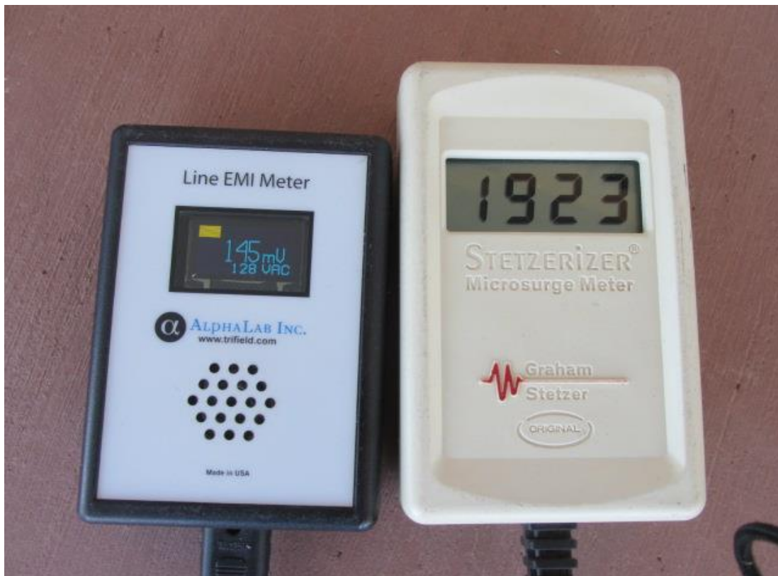
Instruments from Stetzer Electric and Alpha Labs showing high levels of dirty electricity from a sinewave inverter.
