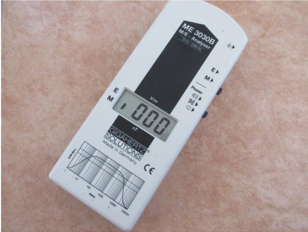
*Instrument that can measure both the electric and the magnetic fields from household wiring. This instrument is sensitive down to 0.01 milligauss (1 nanotesla). It is pictured inside an ultra-low EMF house where the magnetic field is about 0.001 milligauss, so the instrument is unable to detect anything.*
