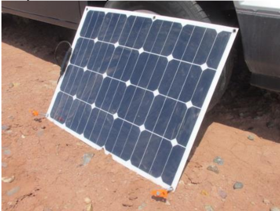
A flexible solar panel is thin and lightweight, but may need to be staked into the ground.
