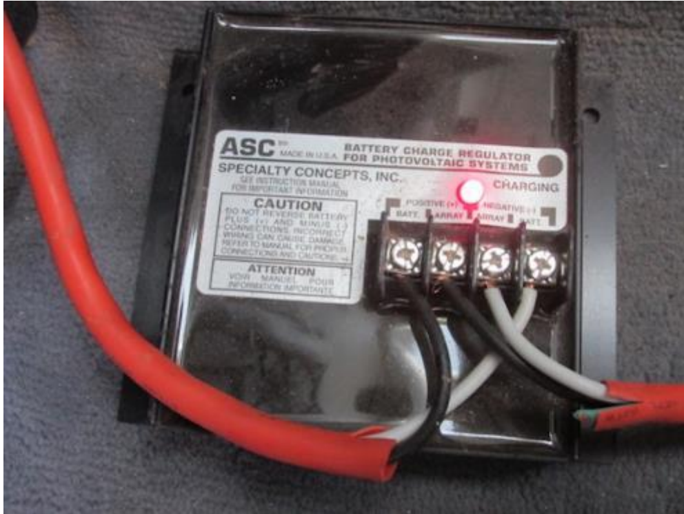
A simple solar charge controller of the brand ASC. It emits virtually no EMF, unlike models with more features.
