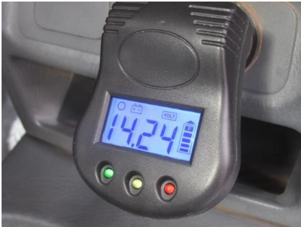
A voltmeter that plugs into a 12 volt socket is an easy way to monitor the battery.
