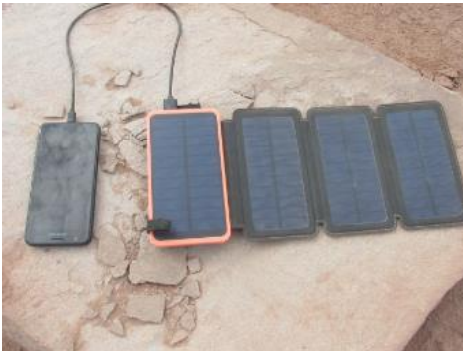
Charging a mobile phone using tiny foldable solar panels.
