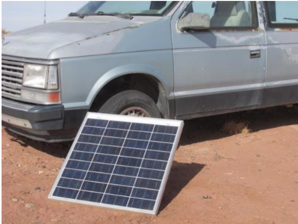
A moveable solar panel is simple and works well if the van isn't moved every day. Here is a framed type panel of 60 watts.
