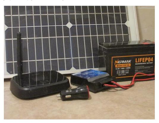
Components for a solar-powered fixed wireless phone system that can be placed well away from the house. The shown T2000 transmitter needs electricity at 5 volts, so a 12to-5 volt USB converter is also shown in the picture. The LVP2 runs directly on 12 volts.
