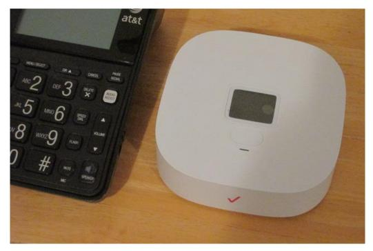
*The model LVP2. It has an internal antenna and no antenna jack for an external antenna. But the backup battery does not have to be in place for it to work.*
