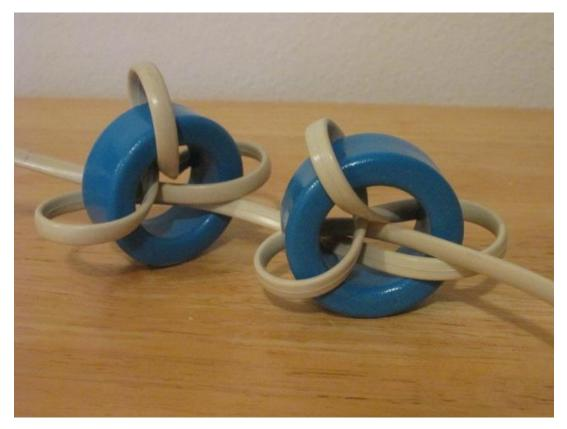
Optional ferrites placed on the cable between the transmitter and the telephone to absorb dirty electricity. Multiple loops of the cable around each ferrite is best. This is an illustration, for best effect make the loops tight around the ferrites.
