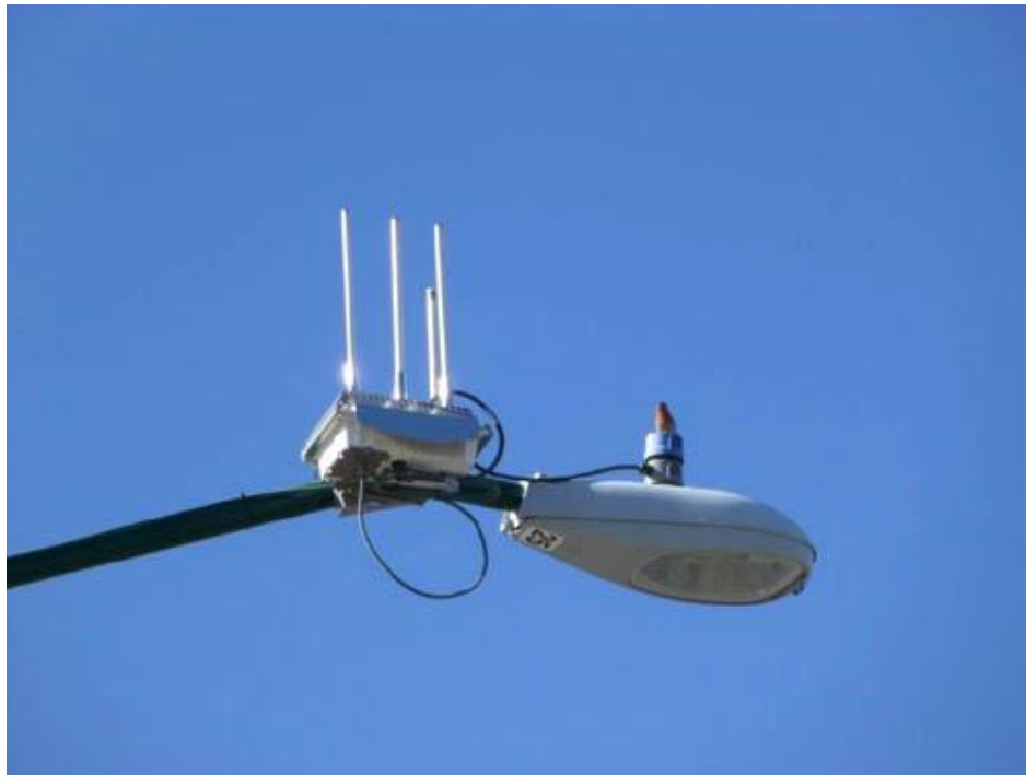
Wireless smart meter communication hub on a lamp post in downtown Phoenix.
