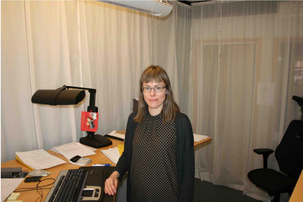
The shielding was done using the Swiss Shield shielding fabric, which is made from threads of copper and silver. The fabric was hung from metal rods attached to the ceiling on all four sides of Veronica. The fabric covered the walls, window and door (see pictures). A slit in the fabric allowed access through the door. The ceiling was shielded with thin aluminum blankets that were mounted underneath the ceiling tiles. The floor was not shielded as there was nothing below the room.
