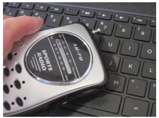
Testing a laptop computer with an AM radio
