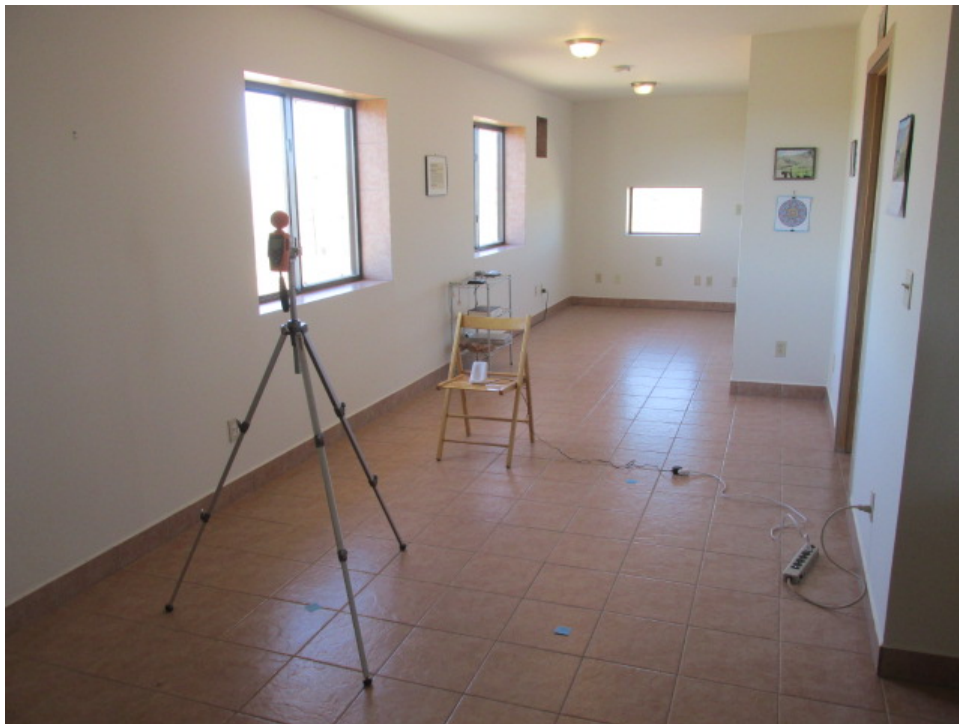
Testing inside House-2. The three big windows (two shown) have no metal-coated glass. The small window has metal low-E coated glass. The tripod is in position A.
