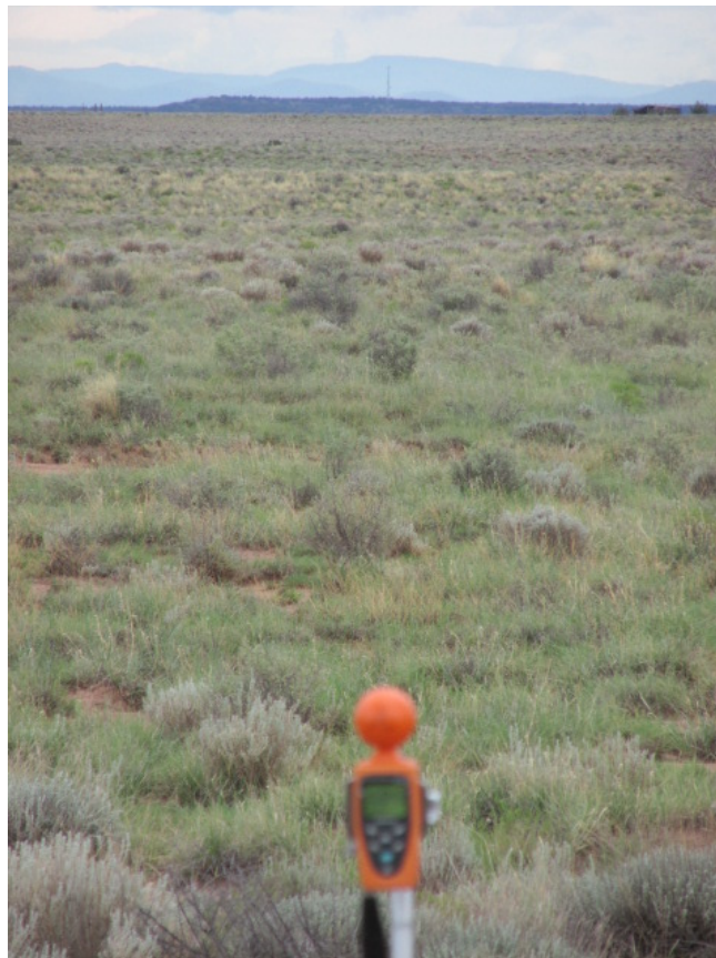
The RF meter on tripod in the yard with cellular base station on top of the dark hill, 10 miles (16 km) away.
