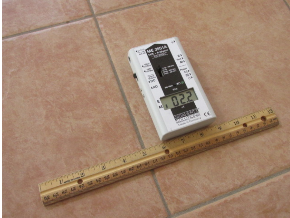
Measuring magnetic fields in the 5 Hz to 400 kHz range at Position D. The pipe embedded in the concrete floor goes between the bottom and the top of the picture.
