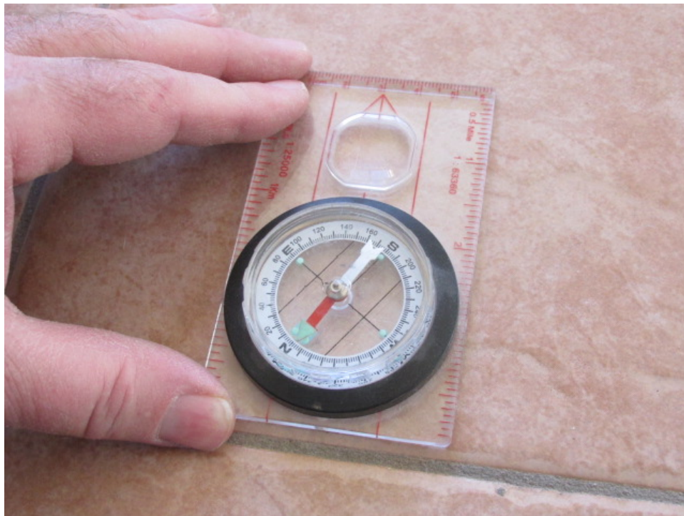
Checking DC magnetic fields with a compass.
